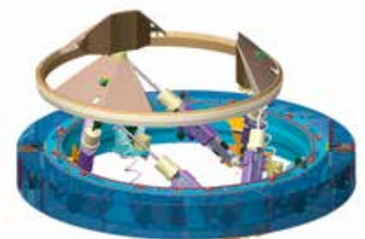
Top An artist's impression of the Dreamchaser docked at the ISS. Bottom The IBDM system with its rigid inner ring and flexible outer ring.
