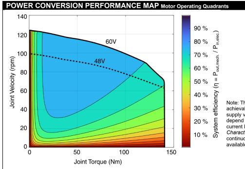
Note: This graphic shows the maximum achievable joint torque/velocities for the given supply voltages. Continuous operating points depend on system cooling and DC link input current limits. Refer to the *Power Conversion Characteristics* table above for potential feasible continuous operating points. Further details are available upon request.
